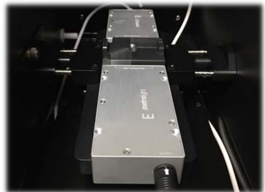
FIGURE 3: P4350 Laser Micrometer (mounted inside the Evo 220)
